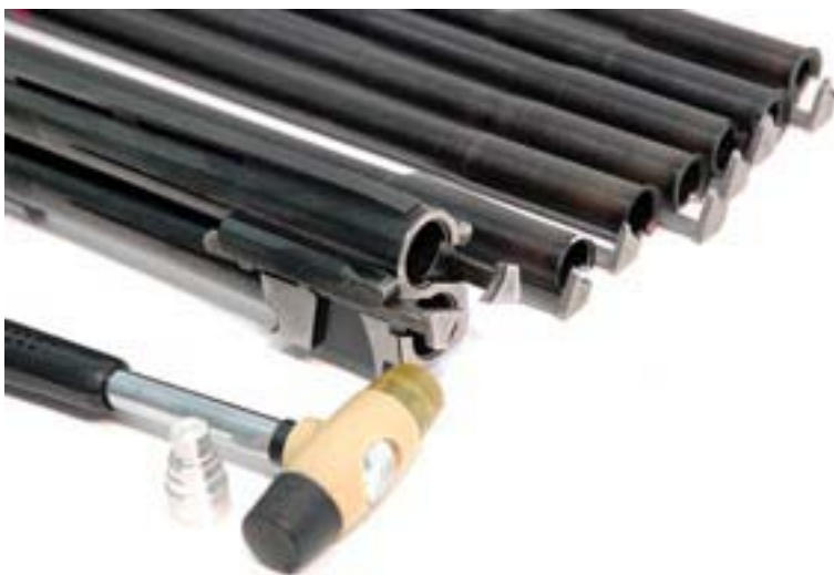
Purbaugh System with tubes, ejectors, plug & hammer.
